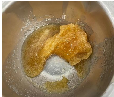
Figure 3.2 - Paste formation after 20% MH incorporation into the P40 ink. A heterogeneous and non-printable paste was formed.
