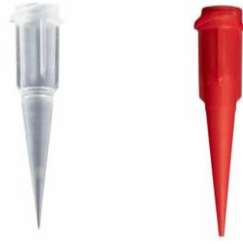
Figure 2.2 - Plastic nozzles used for printing of the 3D hydrogel inks. The red and white nozzles are tapered plastic tips with 25 Gauge and an inner diameter of 0.250 mm and 27 Gauge and an inner diameter of 0.200 mm, respectively. Pictures retrieved from [66].
